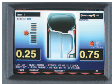
Screen on a typical balancer prior to lowering the hood for automatic measurement.
