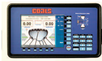
Screens with newer balancers show inboard and outboard measurements automatically.
