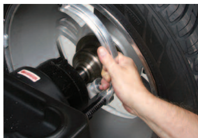
A view of the pressure monitoring sensor being placed on the rim of the wheel.
