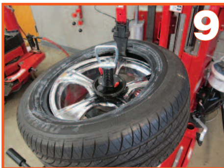
Use the changer's lever to slip the top head over the rim flange.
