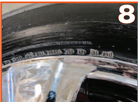
8 Identify the maximum air pressure for the tire. You will need that information to properly seat both beads using air pressure.
