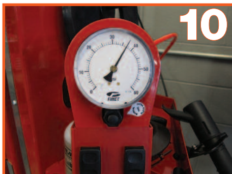
10 Find the proper inflation pressure for the tires on the vehicle placard located in the driver's door jamb or the vehicle owner's manual. Inflate the tire to that pressure. For uniformity, deflate and then inflate again.
