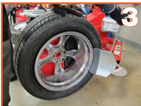
Use breaking shovel to unseat the top bead.
