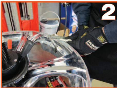
Remove old rubber valve stem, being careful to not damage the wheel. This particular tool breaks the rubber stem into two pieces; make sure to remove the other piece from inside the drop center of the wheel.
