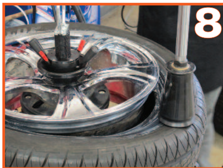
Break top head by pushing down using the changer's unique tool.
