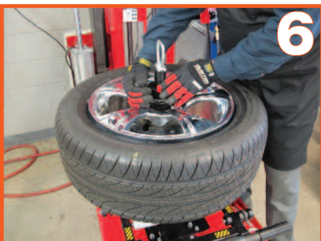
Here the assembly is being mounted on a center post style changer. Make sure to properly position the assembly on the center post when using that type of changer.
