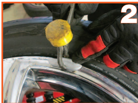
Remove any wheel weights, again being careful not to damage wheel.
