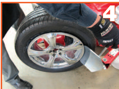
Turn tire/wheel assembly around and repeat using the shovel.
