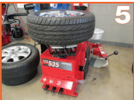
Secure assembly on tire changer. In this photo, the assembly is on a tabletop or rim clamp style changer.
