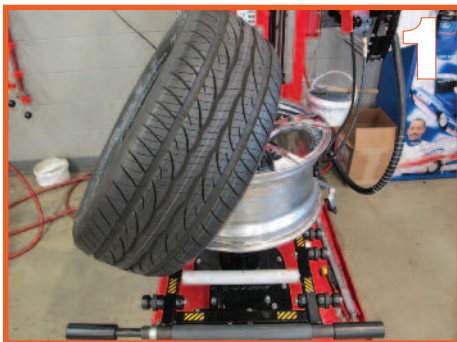
Make sure the tire size matches the wheel diameter and width. After securing wheel to changing machine, check wheel for damage of any type. Also double check to see if the tire has a directional tread.
