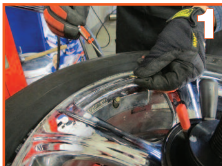
After positioning wheel assembly on tire changer, remove valve core. (Note core in technician’s fingers.)
