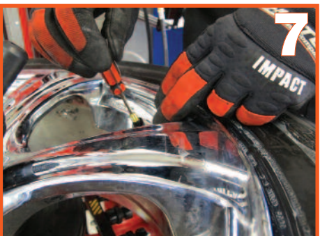
7 Install a new valve core.
