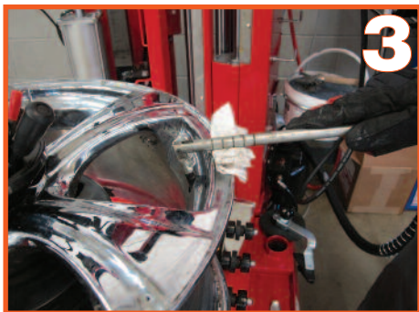
3 Install a fresh rubber valve stem, again taking care to not damage the wheel.
