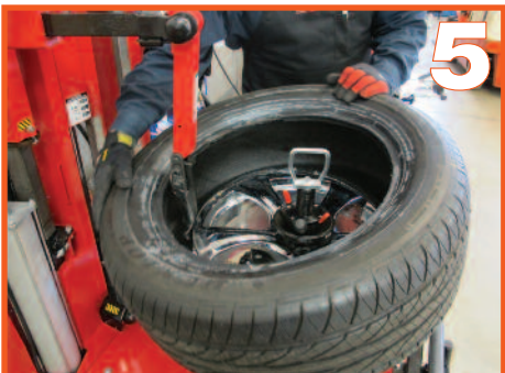
5 Place tire on wheel and with a lever securely in place, twist the tire head over the top rim flange by hand.
