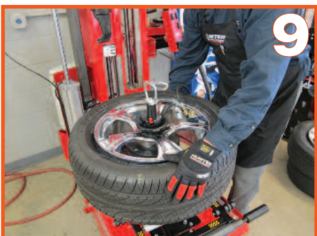
9 Seat both beads using air pressure and a gentle lift of the tire up into the top rim flange.
