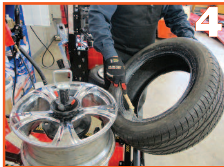
4 Lubricate the inboard and outboard bead areas.
